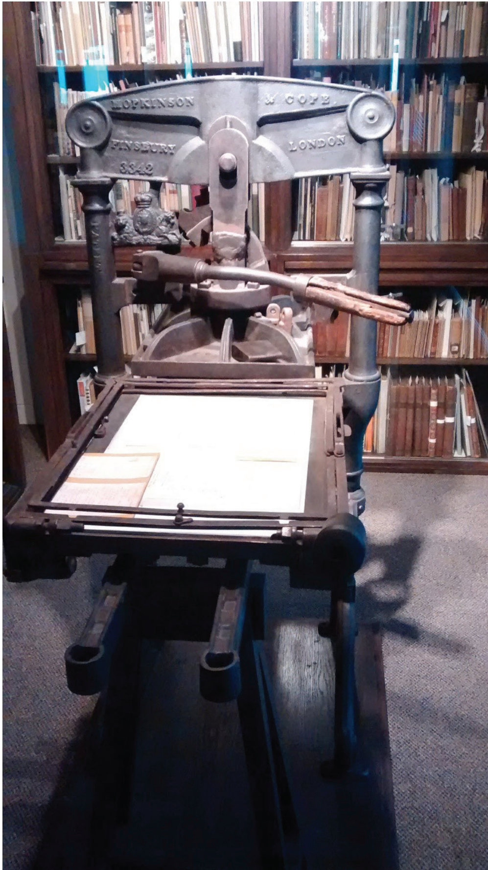
Figure 2: Nineteenth-century single-pull Albion Cree Press. Rare Books and Special Collections, McGill University Library. Photo by Gloria Bell.
